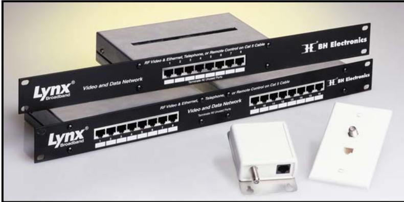
A Lynx distribution hub converts a coaxial television signal into eight UTP output signals that travel on pair four of the UTP cables. It also delivers Ethernet on pairs two and three. At the point of use, the television signals are converted back to coaxial form and the data signals are delivered to an RJ-45 connector.
